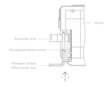
Ensure that the extension arm is fitted securely.
